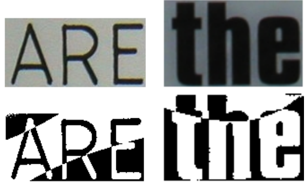
Figure 4: Sample segmentations that result from poor initialization using a mixture of two regressions.
