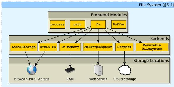
**Figure 2.** An overview of the DOPPIO file system. Much like an actual operating system, DOPPIO’s architecture decouples the frontend interface that programs interact with from the backend implementation that is responsible for interfacing with a particular type of persistent storage.
