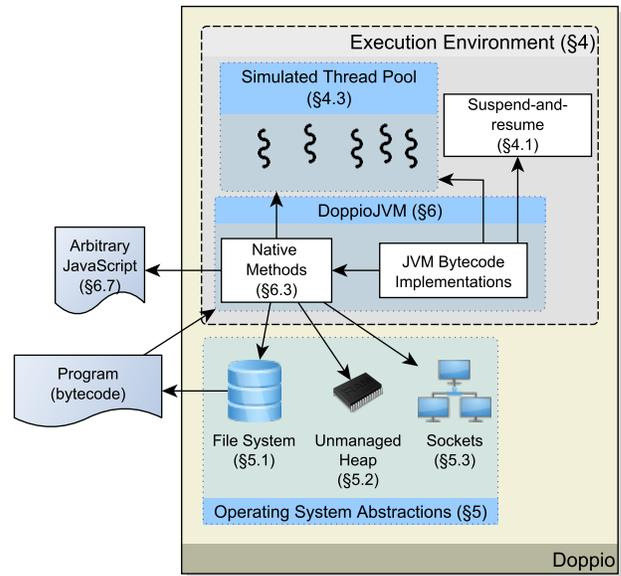
**Figure 1.** The DOPPIO runtime system makes it possible for existing programs to execute in an unmodified browser via its virtualized execution environment and operating system abstractions. This diagram displays the various components of DOPPIO at a high level, and illustrates how language implementations, such as DOPPIOJVM, rely on them.
