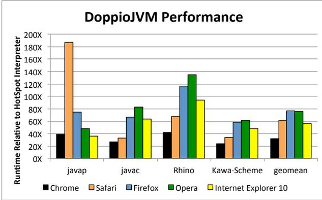
**Figure 3.** DOPPIOJVM’s performance on our benchmark applications relative to the HotSpot JVM interpreter bundled with Java 6. DOPPIOJVM runs between  $24\times$  and  $42\times$  slower (geometric mean:  $32\times$ ) than the HotSpot interpreter in Google Chrome. Note that javap’s poor performance in Safari is due to a browser bug; we discuss this further in Section 7.
