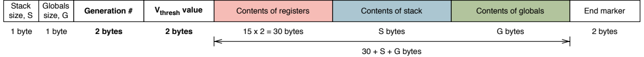
Figure 3.8. A state checkpoint in the adaptive version of Mementos. As in the non-adaptive version, the length of the entire checkpoint can be calculated from the two-byte header. Mementos uses an additional four bytes of metadata (shown in bold) to decide whether to adjust its checkpointing voltage threshold V_{\text{thresh}} up or down.
