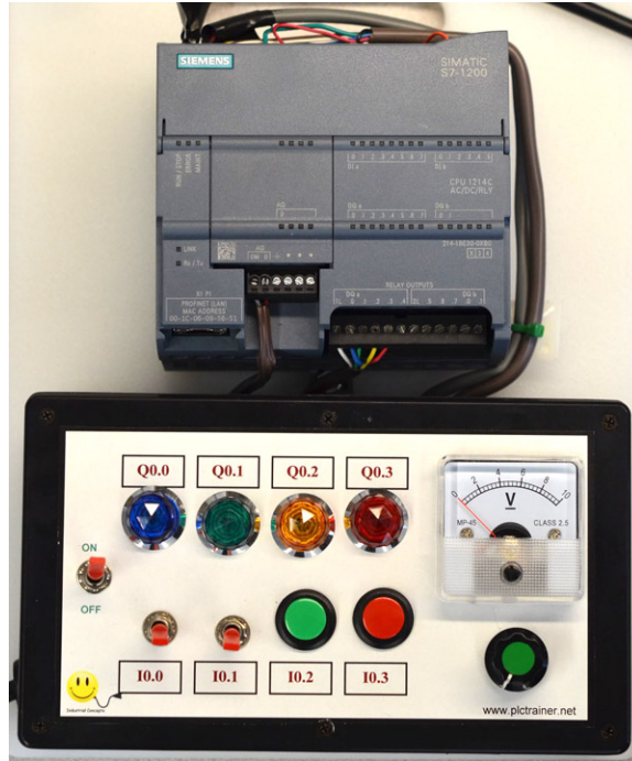
Figure 3.1: A Siemens S7-1200 1214C AC/DC/Rly PLC (top) with a “trainer” box providing input and output hardware (bottom).
