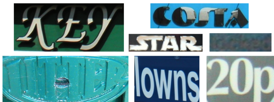
Figure 7.4: Sample images that we recognize incorrectly. Characteristics that make these images difficult include low resolution, abrupt lighting changes and low contrast. In addition, words that do not appear in the web-based lexicon, but look similar to something that does can be confused. Here ‘lowns’ is recognized as ‘Towns’ and ‘20p’ is recognized as ‘200’. This image is best viewed in color.
