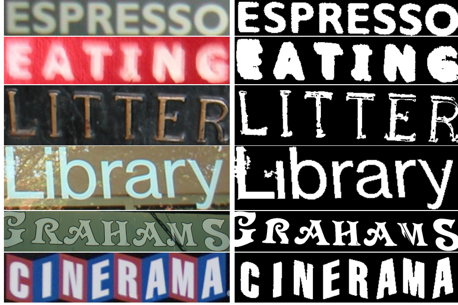
Figure 6.7: Examples of words that we identify correctly and their foreground segmentations.
