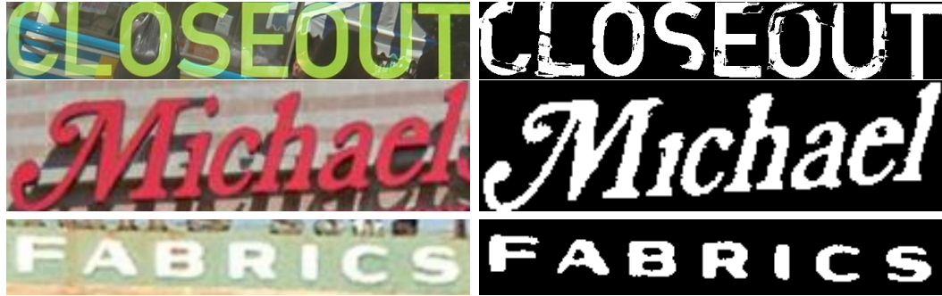
Figure 6.2: Sample images with complex backgrounds and their segmentations using bilateral regression.
