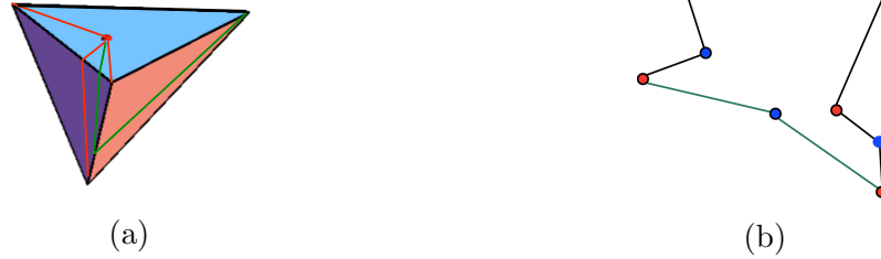
Figure 4.3: (a) One of the shortest paths on the tetrahedron from Fig. 1.3(a) is replaced by a geodesic. (b) The corresponding geodesic star unfolding polygon. Red and blue vertices are source images and polyhedral vertices respectively. One source angle is larger than \pi .
