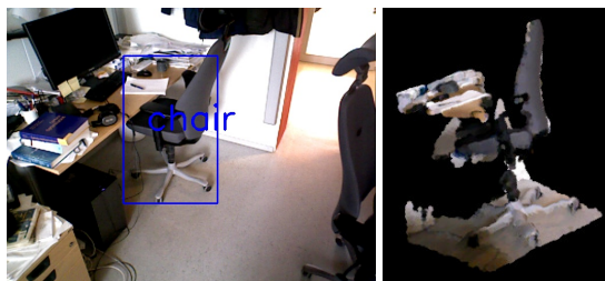
Figure 7: Processing steps of CNN-based object detection. Left: Detect object candidate. Right: Extract partial view.
