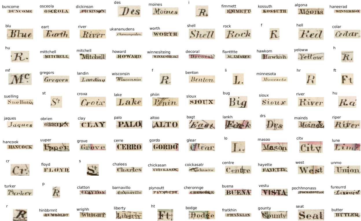
Figure 7. Empirical Results showing the text recognition results based on the fine-tuned CNN using synthetic map training data. Results for map D0042-1070007.
