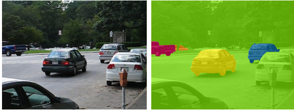
Figure 1.2: Motion segmentation. Every pixel is given one of k labels: k is the number of independently moving objects and static environment. Left to right: original image, motion segmentation
