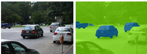
Figure 1.1: Binary motion segmentation. Every pixel is given one of two labels: static environment or moving objects. Left to Right: original image, correct binary segmentation
