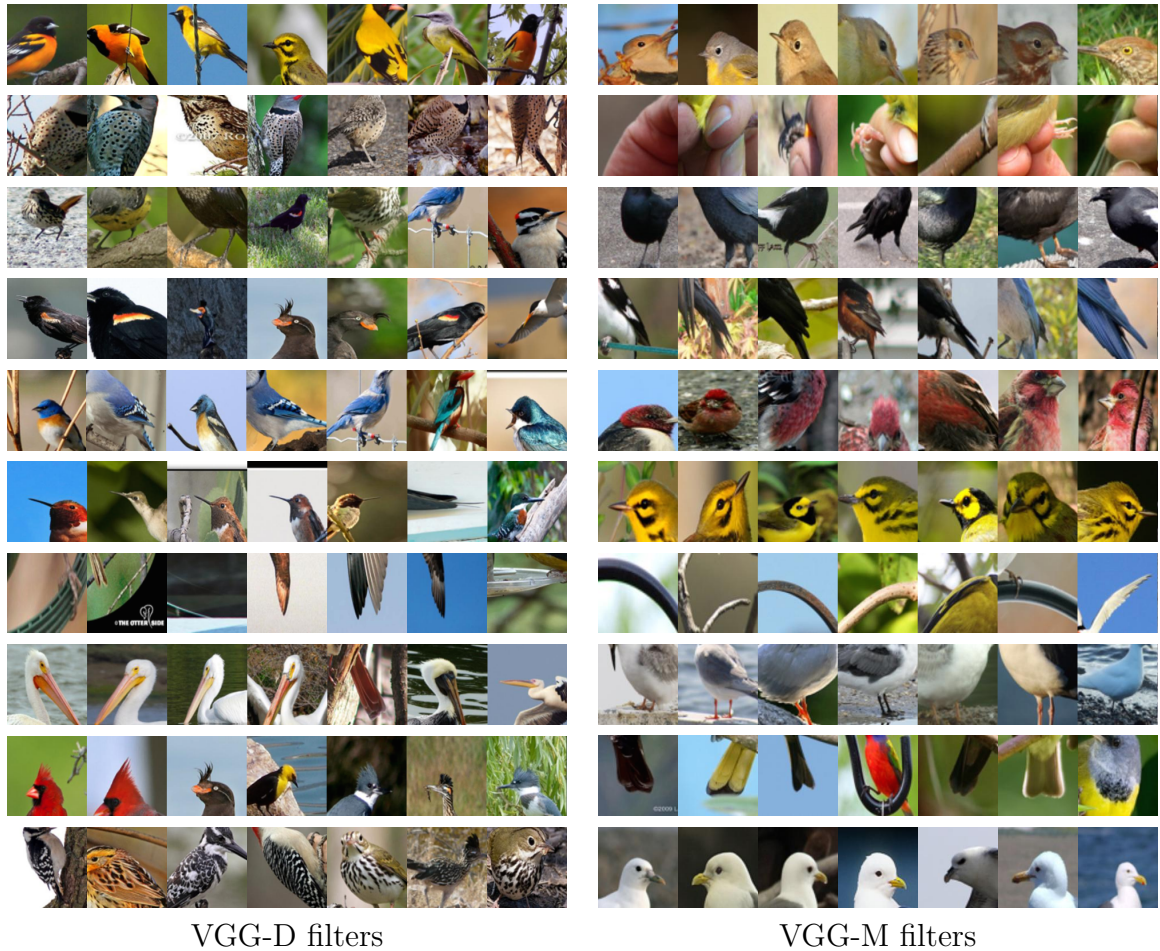
Figure 5.6. Patches with the highest activation for several filters of the fine-tuned B-CNN (VGG-D + VGG-M) model on birds dataset. These visualizations indicate that network units activate on highly localized attributes of objects that capture color, texture, and shape patterns.
