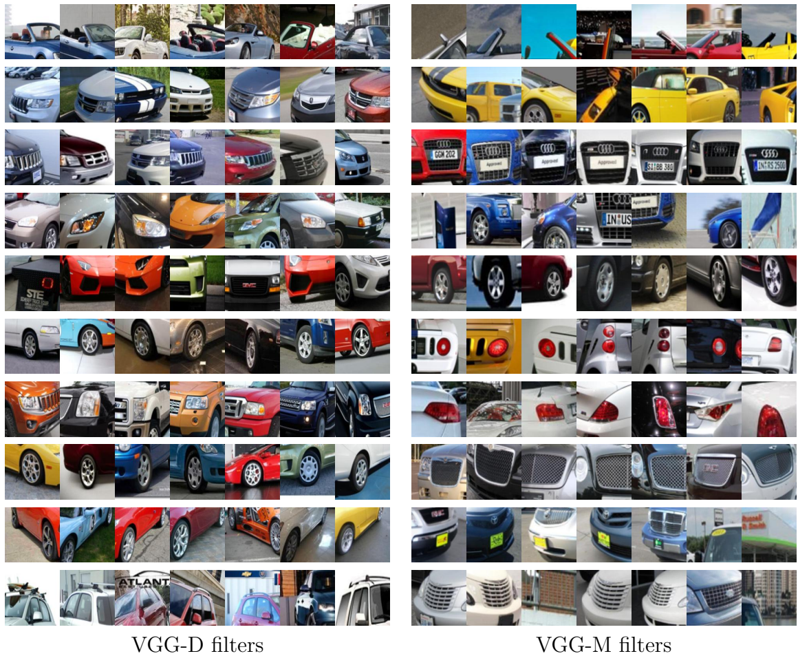
Figure 5.8. Patches with the highest activation for several filters of the fine-tuned B-CNN (VGG-D + VGG-M) model on cars dataset. These visualizations indicate that network units activate on highly localized attributes of objects that capture color, texture, and shape patterns.
